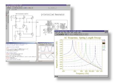
Modeling Tools: MEMS Modeler automatically generates behavioral models ready for system simulation with electronics and packaging from 3D
